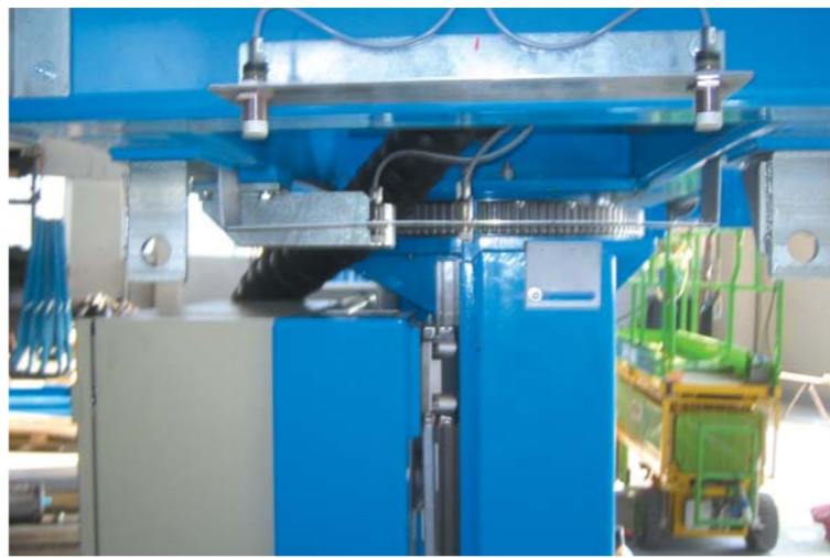
Detail of the rack and screw mechanism of the bridge crane
